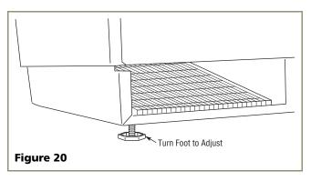
Check the levelness after each adjustment and repeat the previous steps until the unit is level. Go on to 8 Install the Unit.
